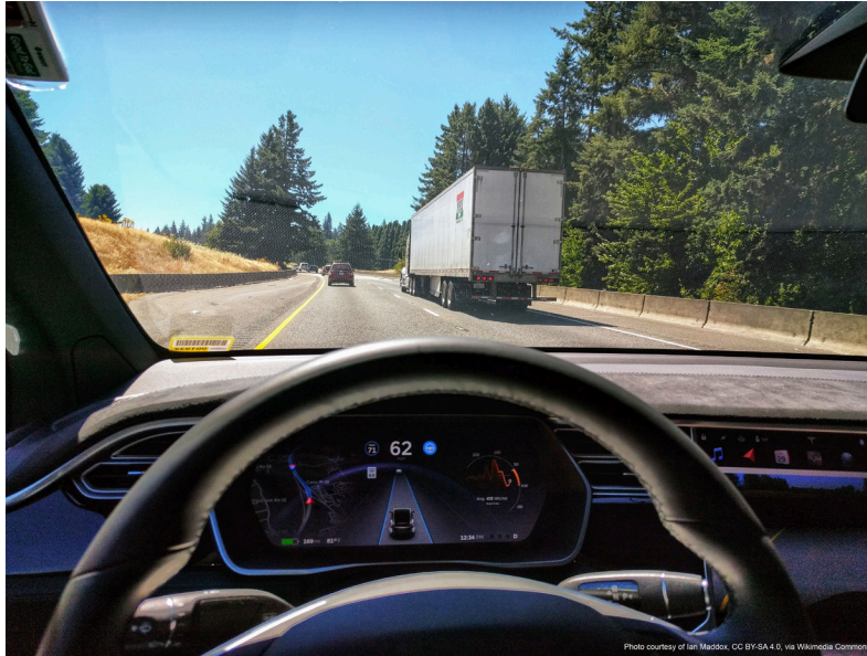
A Tesla Model X engaged in autopilot mode, controlling distance from lead car and centering vehicle in lane
